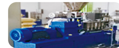
φ26 三螺杆 (倒三角) Tri-screw (inverted triangle)
